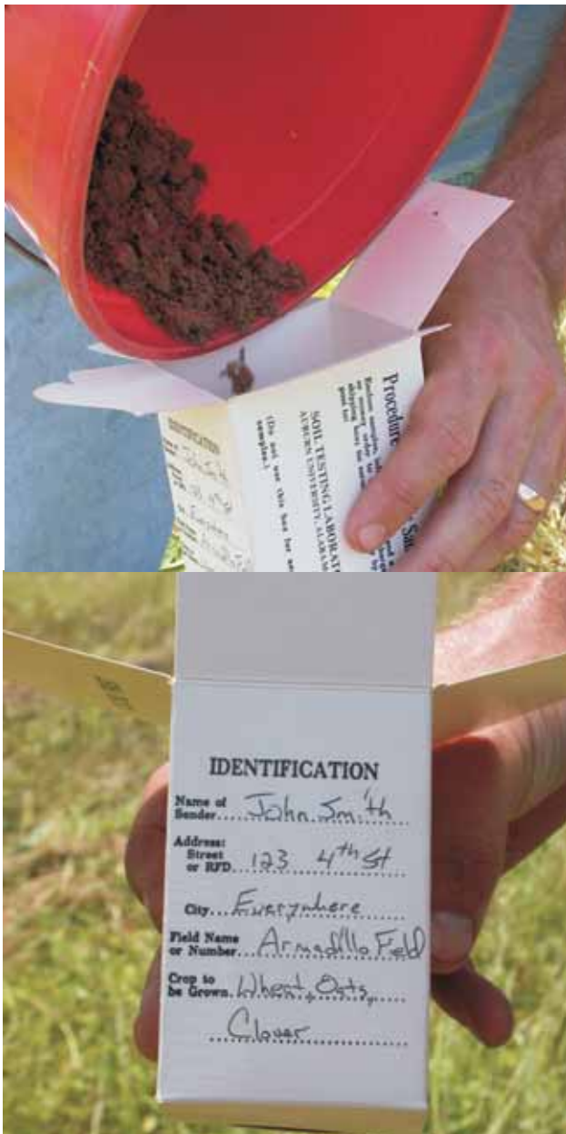
Mix the subsamples and then take one sample from the mixed subsamples (top photo). Make sure each soil sample is properly labeled with the food plot's name and the crop to be planted before sending it to the soil-testing lab (bottom photo). CHRIS COOK
