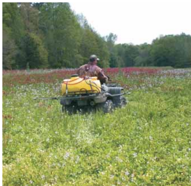
An ATV equipped with a boom sprayer is ideal for applying herbicides to most one-acre or smaller food plots.
