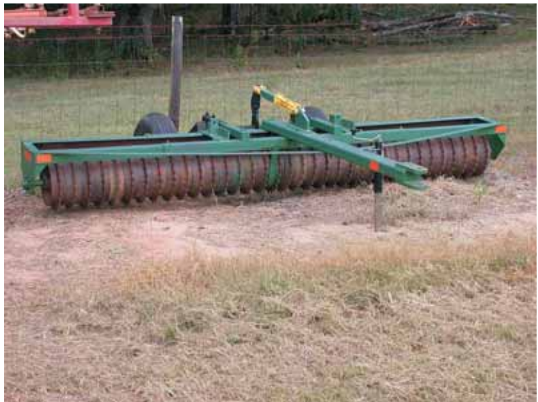
A culti-packer is one of the best ways to cover seed after planting. This implement also does a great job of preparing a firm, smooth seed bed after plowing.
